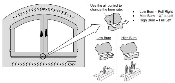
**Warning:** The air control becomes hot during operation - use gloves or a tool to prevent burns.
